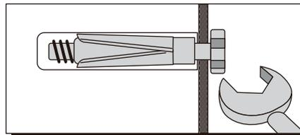
For use with heavier loads such as TV & HiFi Speakers and Satellite Dishes etc.
