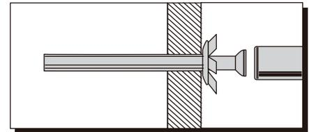
For use with walls stuck with plaster board. The hammer fixing allows it to be fixed to the wall rather than the plaster board. Always check the fixing is secure to the retaining wall.
