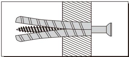
Generally aerated blocks should not be used to support heavy loads, use a specialist fitting in this case. For light loads, a General Purpose Plug can be used.
