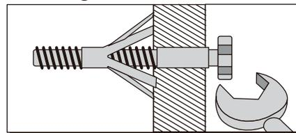
For use when fitting or supporting heavy loads such as shelving, wall cabinets, coat racks.
